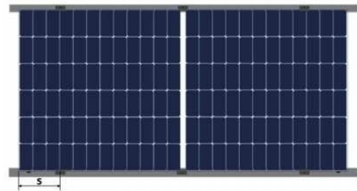
Installation of frameless module with fixtures on long sides (clamp length = 150mm)
